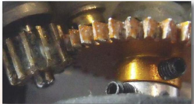
*Initially applied lubrication dries to a white coverage*
